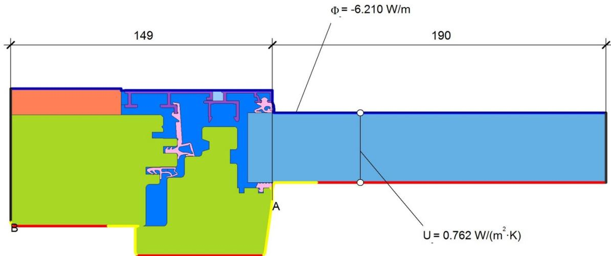
$$U_{f,A,B} = \frac{\frac{\Phi}{\Delta T} - U_p \cdot b_p}{b_f} = \frac{\frac{6.210}{20.000} - 0.762 \cdot 0.190}{0.149} = 1.112 \text{ W/(m}^2 \cdot \text{K)}$$
