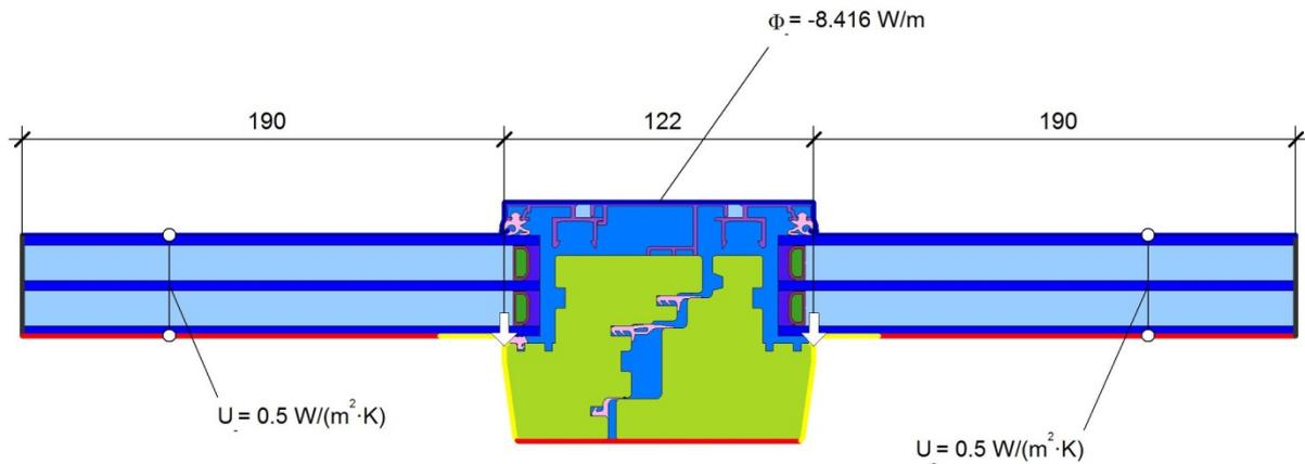
$$\psi = \frac{\Phi}{\Delta T} = \frac{U_{g1} \cdot b_{g1} + U_f \cdot b_f + U_{g2} \cdot b_{g2}}{2} = \frac{0.500 \cdot 0.190 + 1.291 \cdot 0.122 + 0.500 \cdot 0.190}{2} = 0.037 \text{ W/(m} \cdot \text{K)}$$
