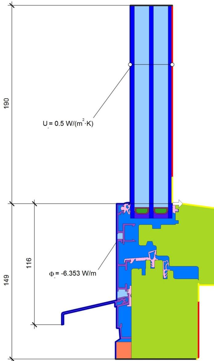
$$\psi = \frac{\Phi}{\Delta T} - U_g \cdot b_g - U_f \cdot b_f = \frac{6.353}{20.000} - 0.500 \cdot 0.190 - 1.249 \cdot 0.149 = 0.037 \text{ W/(m}\cdot\text{K)}$$
