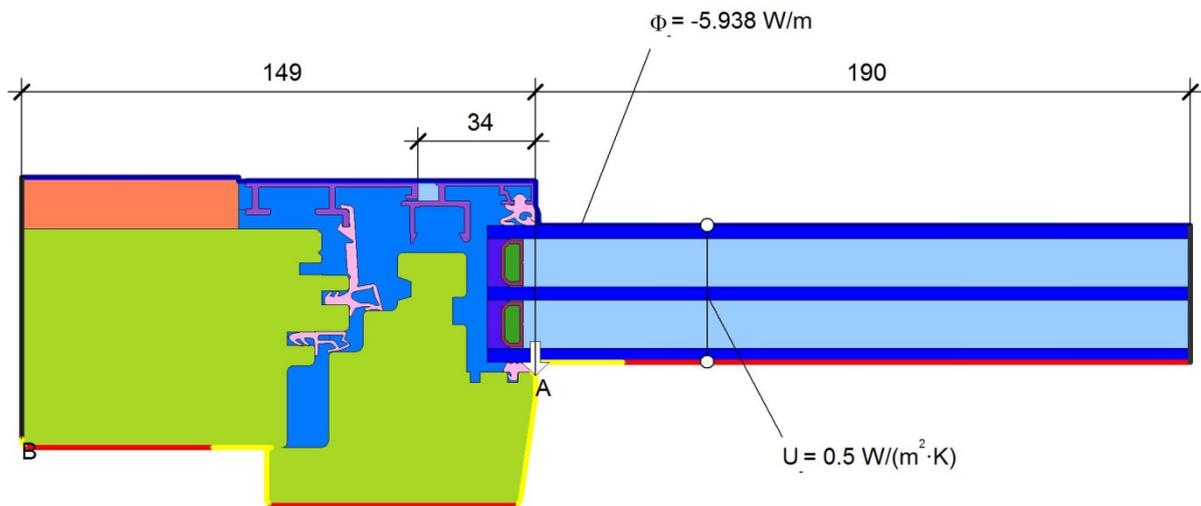
$$\psi_A = \frac{\Phi}{\Delta T} - U_g \cdot b_g - U_f \cdot b_f = \frac{5.938}{20.000} - 0.500 \cdot 0.190 - 1.112 \cdot 0.149 = 0.036 \text{ W/(m}\cdot\text{K)}$$
