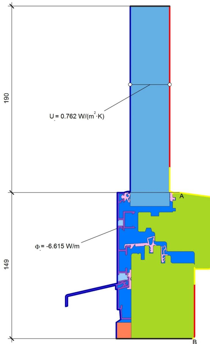
$$U_{f,A,B} = \frac{\frac{\Phi}{\Delta T} - U_p \cdot b_p}{b_f} = \frac{\frac{6.615}{20.000} - 0.762 \cdot 0.190}{0.149} = 1.249 \text{ W/(m}^2 \cdot \text{K)}$$
