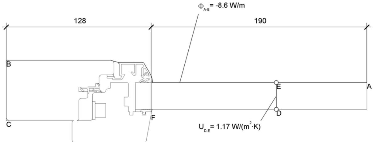
$$U_{fF} = \frac{\frac{\Phi}{\Delta T} - U_p \cdot b_p}{b_f} = \frac{\frac{-8.645}{-20.000} - 1.169 \cdot 0.191}{0.128} = 1.638 \text{ W/(m}^2 \cdot \text{K)}$$
