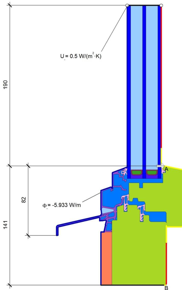
$$\psi_A = \frac{\Phi}{\Delta T} - U_g \cdot b_g - U_f \cdot b_f = \frac{5.933}{20.000} - 0.500 \cdot 0.190 - 1.172 \cdot 0.141 = 0.036 \text{ W/(m} \cdot \text{K)}$$
