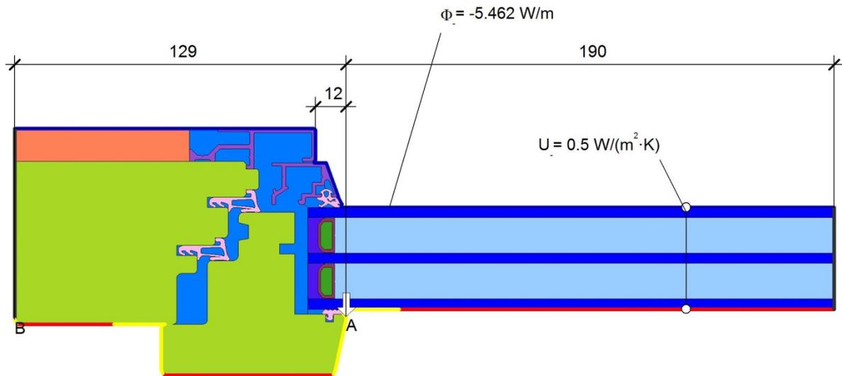
$$\psi = \frac{\Phi}{\Delta T} - U_g \cdot b_g - U_f \cdot b_f = \frac{5.462}{20.000} - 0.500 \cdot 0.190 - 1.107 \cdot 0.129 = 0.035 \text{ W/(m} \cdot \text{K)}$$
