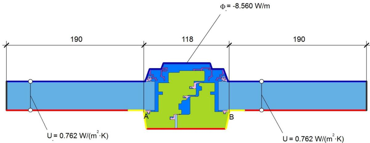
$$U_{fA,B} = \frac{\frac{\Phi}{\Delta T} - U_{p1} \cdot b_{p1} - U_{p2} \cdot b_{p2}}{b_f} = \frac{\frac{8.560}{20.000} - 0.762 \cdot 0.190 - 0.762 \cdot 0.190}{0.118} = 1.174 \text{ W/(m}^2 \cdot \text{K)}$$
