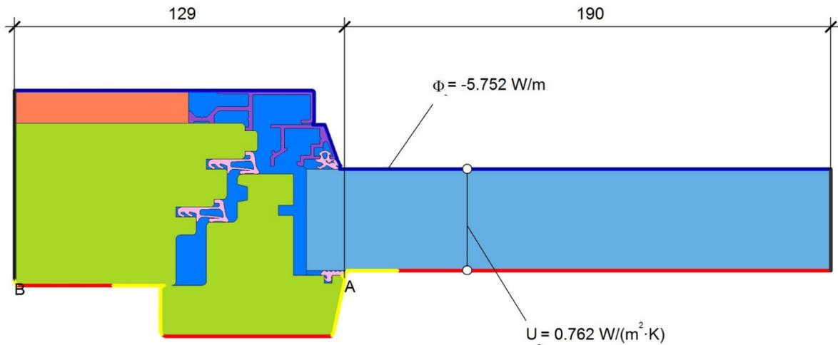
$$U_{fA,B} = \frac{\frac{\Phi}{\Delta T} - U_p \cdot b_p}{b_f} = \frac{\frac{5.752}{20.000} - 0.762 \cdot 0.190}{0.129} = 1.107 \text{ W/(m}^2 \cdot \text{K)}$$
