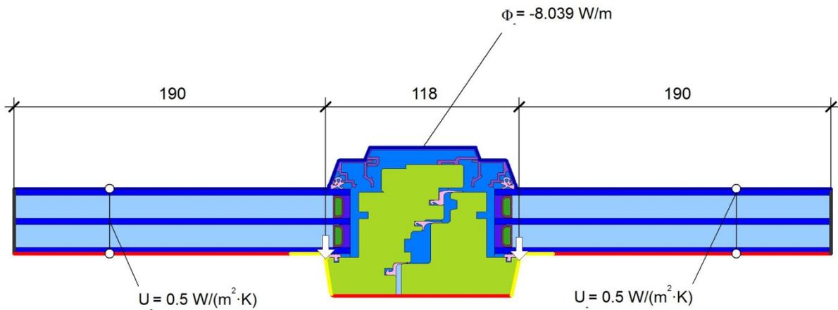
$$\psi = \frac{\Phi}{\Delta T} - \frac{U_{g1} \cdot b_{g1} - U_f \cdot b_f - U_{g2} \cdot b_{g2}}{2} = \frac{8.039}{20.000} - \frac{0.500 \cdot 0.190 - 1.174 \cdot 0.118 - 0.500 \cdot 0.190}{2} = 0.037 \text{ W/(m} \cdot \text{K)}$$
