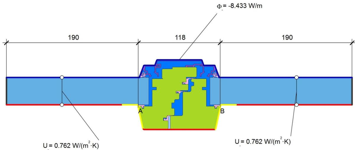
$$U_{f,A,B} = \frac{\frac{\Phi}{\Delta T} - U_{p1} \cdot b_{p1} - U_{p2} \cdot b_{p2}}{b_f} = \frac{\frac{8.433}{20.000} - 0.762 \cdot 0.190 - 0.762 \cdot 0.190}{0.118} = 1.120 \text{ W/(m}^2 \cdot \text{K)}$$
