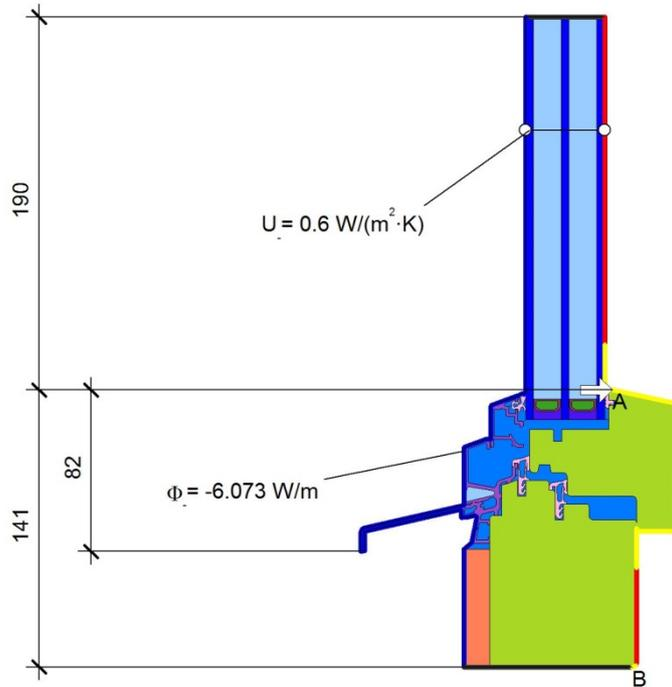
$$\psi_A = \frac{\Phi}{\Delta T} - U_g \cdot b_g - U_f \cdot b_f = \frac{6.073}{20.000} - 0.600 \cdot 0.190 - 1.094 \cdot 0.141 = 0.035 \text{ W/(m} \cdot \text{K)}$$
