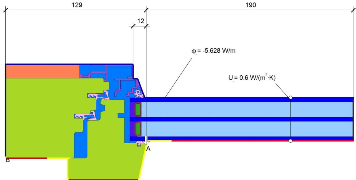
$$\psi_A = \frac{\Phi}{\Delta T} - U_g \cdot b_g - U_f \cdot b_f = \frac{5.628}{20.000} - 0.600 \cdot 0.190 - 1.035 \cdot 0.129 = 0.034 \text{ W/(m}\cdot\text{K)}$$
