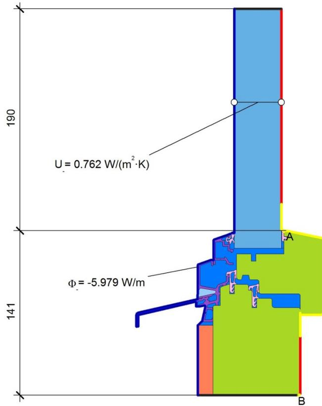
$$U_{f,A,B} = \frac{\frac{\Phi}{\Delta T} - U_p \cdot b_p}{b_f} = \frac{\frac{5.979}{20.000} - 0.762 \cdot 0.190}{0.141} = 1.094 \text{ W}/(\text{m}^2 \cdot \text{K})$$
