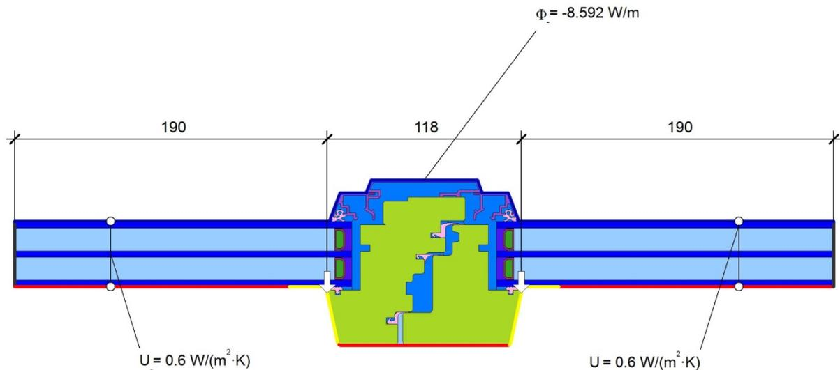
$$\psi = \frac{\Phi}{\Delta T} = \frac{U_{g1} \cdot b_{g1} + U_f \cdot b_f + U_{g2} \cdot b_{g2}}{2} = \frac{0.600 \cdot 0.190 + 1.120 \cdot 0.118 + 0.600 \cdot 0.190}{2} = 0.035 \text{ W/(m} \cdot \text{K)}$$
