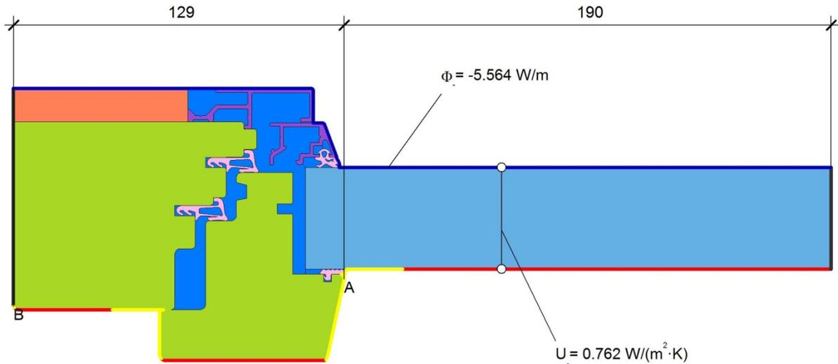
$$U_{fAB} = \frac{\frac{\Phi}{\Delta T} - U_p \cdot b_p}{b_f} = \frac{\frac{5.564}{20.000} - 0.762 \cdot 0.190}{0.129} = 1.035 \text{ W}/(\text{m}^2 \cdot \text{K})$$
